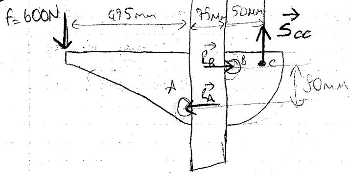
$$\left\{ \begin{array}{l} \vec{S}_{cc}, \vec{R}_A, \vec{R}_B, \vec{F} \end{array} \right\} = 0$$
