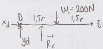
$$\text{denge denklemleri} \begin{cases} \Sigma x_c = 0 \Rightarrow x_D = 0 \\ \Sigma y = 0 \Rightarrow Y_D + R_C - W_1 = 0 \\ \Sigma M_D = 0 \Rightarrow R_C \cdot r - W_1 \cdot \frac{3r}{2} = 0 \end{cases}$$
