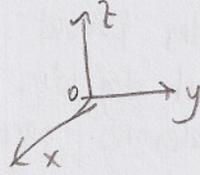
$$\left. \begin{aligned} \sum Z &= 0 \\ \sum M_{0x} &= 0 \\ \sum M_{0y} &= 0 \end{aligned} \right\} \begin{array}{l} 3 \text{ denk.} \\ 3 \text{ bil. çözümler.} \end{array}$$
