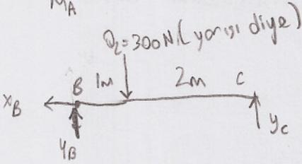
$$\text{BC için } \left\{ \begin{array}{l} \sum X = 0 \Rightarrow X_B = 0 \text{ ve } X_A = 0 \\ \sum Y = 0 \Rightarrow Y_B + Y_C - Q_2 = 0 \\ \sum M_B = 0 \Rightarrow -Q_2 \cdot 1 + Y_C \cdot 3 = 0 \end{array} \right.$$
