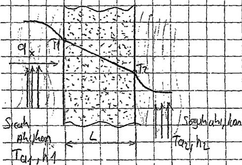
$$q_x'' = h_1 (T_1 - T_2) \Rightarrow q_x = \frac{T_1 - T_2}{\frac{1}{h_1 A} + \frac{L}{k A} + \frac{1}{h_2 A}}$$
